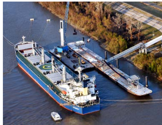
On floating docks, our pedestal-mounted cranes on barge ensure the transfer of bulk materials to a storage area on shore
